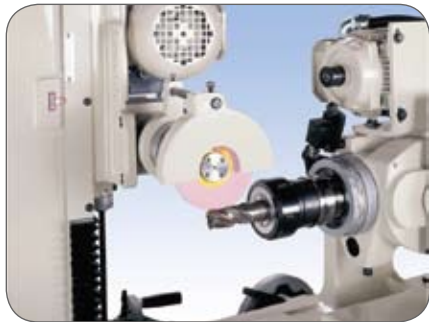
3. Grinding outer diameter
