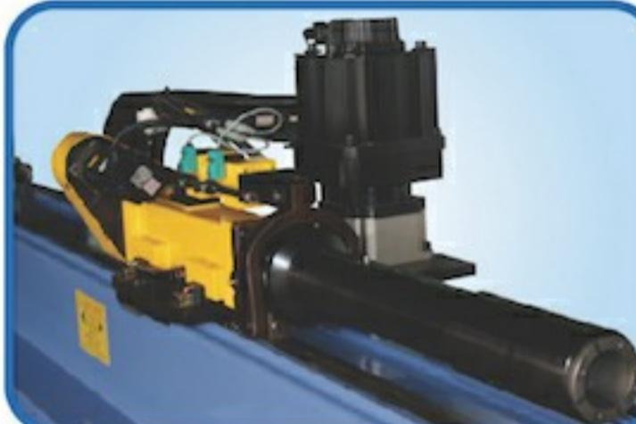
■ The slide ways are mounted with precision linear guide ways.
