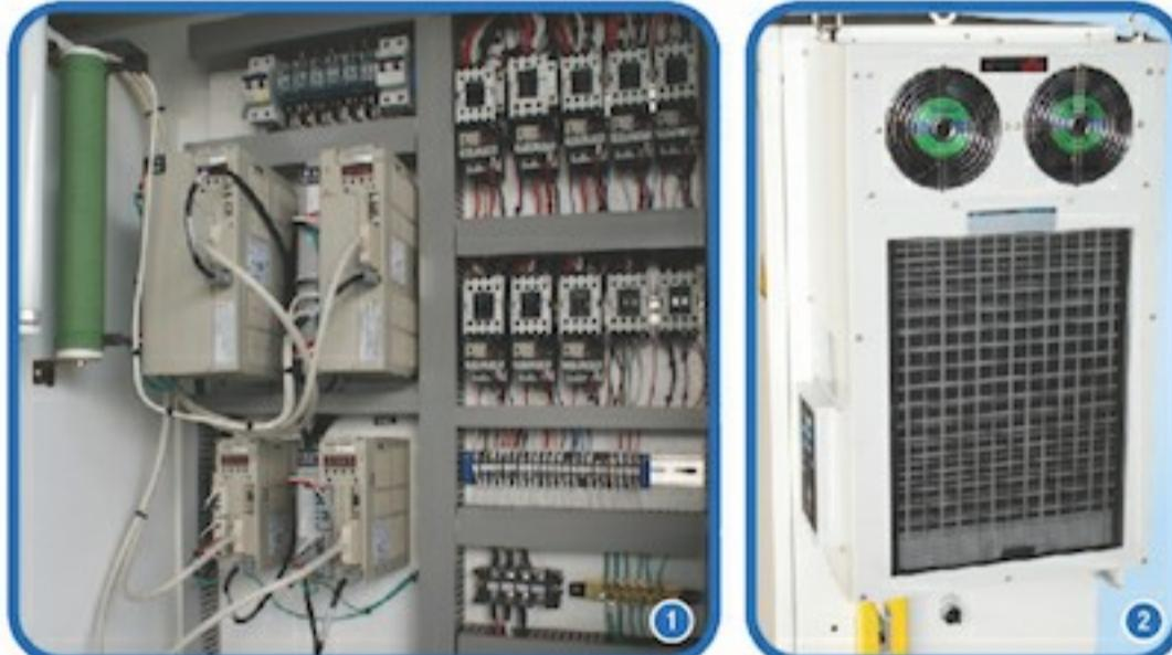
The electrical cabinet is a modular design and is separately mounted from the machine to prevent being affected by machine vibration.
