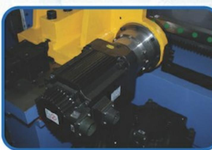
■ Driven by Electric Servo Motor
